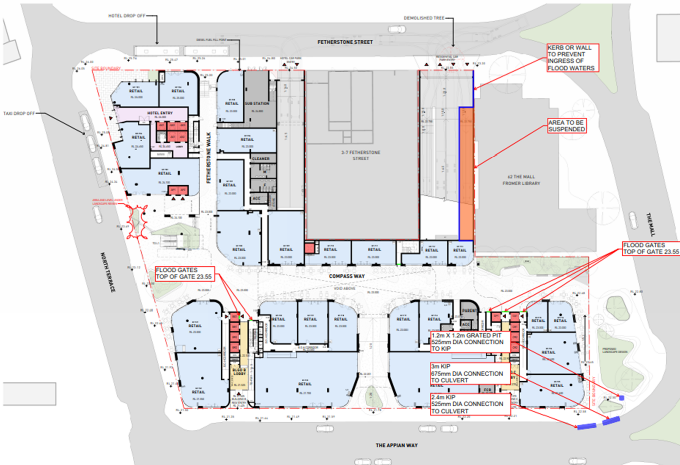
Figure 18 - Flood Protection Measures
